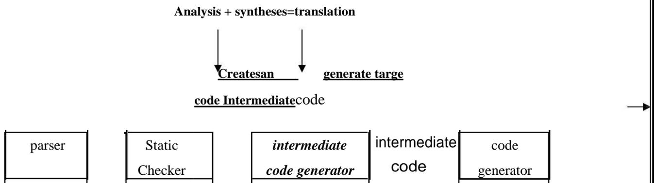
In the analysis –synthesis model of a compiler, the front-end translates a source program into an intermediate representation from which the back-end generates target code, in many compilers the source code is translated into a language which is intermediate in complexity between a HLL and machine code .the usual intermediate code introduces symbols to stand for various temporary quantities.
